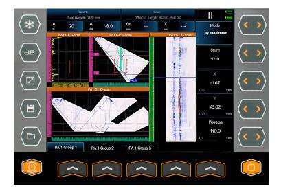
Weld image on the Scan and B-scan based on true beam path give the operator easy understanding of defect location and geometry in the object.
